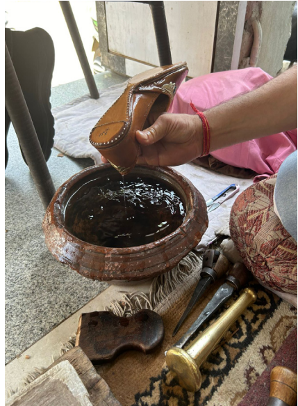
The process of reshaping a worn jutti begins by soaking it in water, allowing the leather to soften and become pliable. Photo by Nandini Agarwal.
