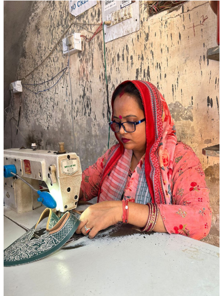
Inside the craftsman’s home, his wife pipes the jutti uppers on a sewing machine with remarkable speed and precision. Photo by Nandini Agarwal.
