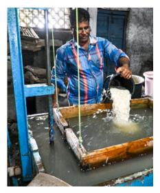
Mohammad Altaf pours the pulp into the frame of the vico vat machine which is operated by hand. Photo by Anil Purohit.
