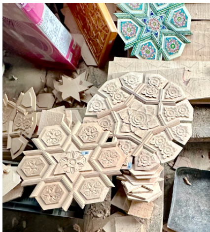
Khatamband ceilings—crafted without nails, featuring interlocking wooden patterns. Photo by Taha Mughal.
